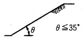
$\theta \leq 35^\circ$ | 崖面の角度が 35 度を超え 45 度以下のもの。<br>
