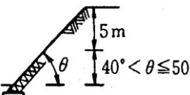
$40^\circ < \theta \leq 50^\circ$ | 崖面の角度が 50 度を超えるもの。<br>
