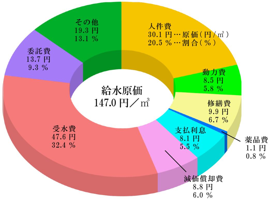
$$\text{給水原価} = \frac{(\text{経常費用} - \text{特別損失}) - (\text{受託工事費} + \text{長期前受金戻入})}{\text{年間有収水量}} = \frac{(35,250,114 \text{千円} - 87,028 \text{千円}) - (155,255 \text{千円} + 4,734,738 \text{千円})}{205,951 \text{千m}^3} = 147.0 \text{円/m}^3$$
