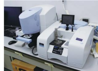
Fourier transform infrared spectroscopy
