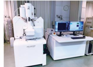
Electron probe micro analyzer(EPMA)
