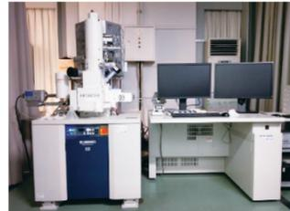
Field emission scanning electron microscope(FE-SEM)
