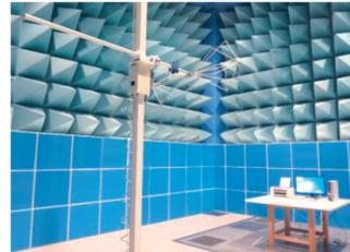
Electromagnetic anechoic chamber
